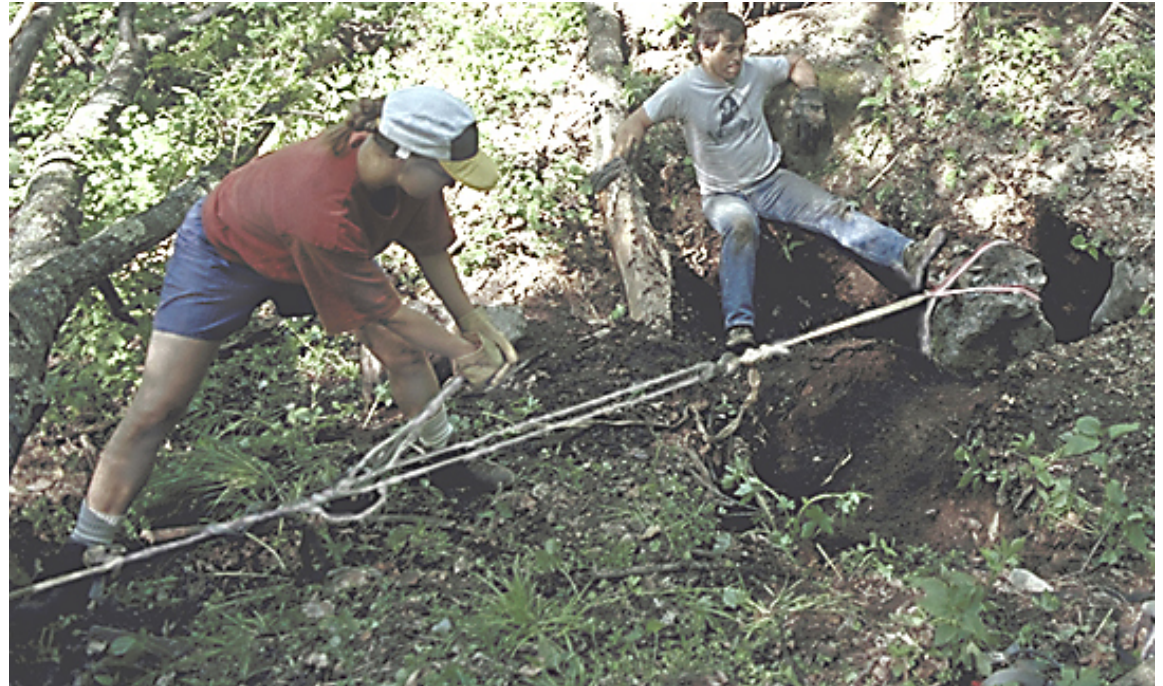
Surface weathering and erosion often plug cave entrances at the land surface. Here cavers relocate a boulder using a ratchet winch, webbing slings and hand tools. The next obstacle was an aid climb; the passage thus gained continues.
